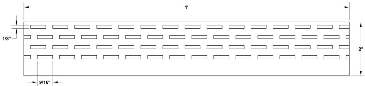
7 sqin of perforated area in a 12" piece of vented ridge. Based on 1/2" x 1/8" holes, 56 per side, with 2 sides.
