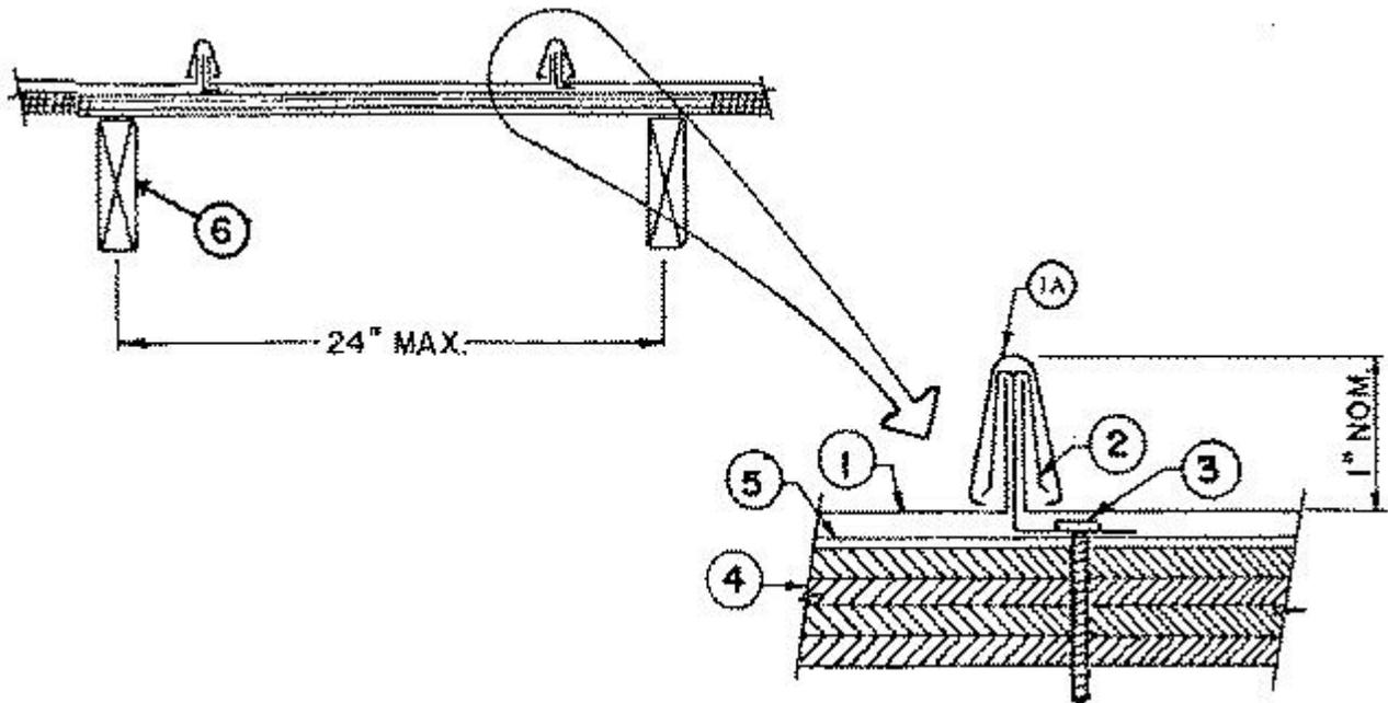
1. **Metal Roof Deck Panels\*** — No. 24 MSG min coated steel. Max panel width 22-3/4 in. Panels continuous over two or more spans. End laps to occur adjacent to supports with panels overlapped 4 in. A line of sealant may be used at panel ends and side laps.
