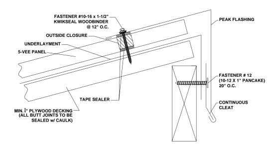
Figure 8: Peak Flashing Detail
