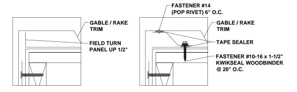
Figure 12: Gable/Rake Detail
