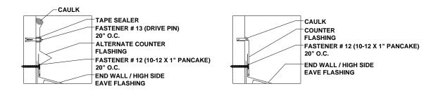
Figure 11: Floating Endwall/Parapet High Side Eave Detail
