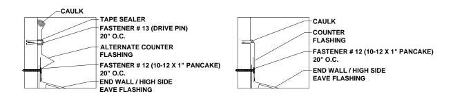
Figure 10: Fixed Endwall/Parapet High Side Eave Detail
