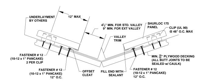
Figure 3: Valley Detail (Valley With Offset Cleat)
