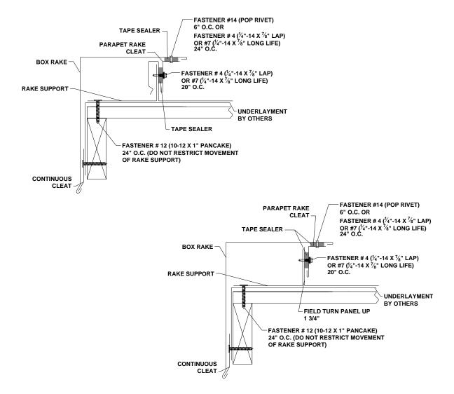
Figure 17: Sidewall/Parapet Floating Rake Flashing Detail
