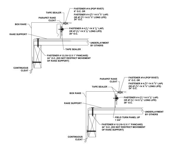
Figure 7: Floating Rake/Gable Flashing Detail
