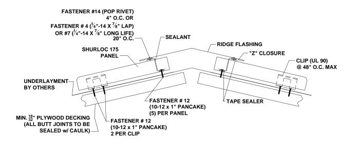
Figure 1: Fixed Ridge/Hip Detail
