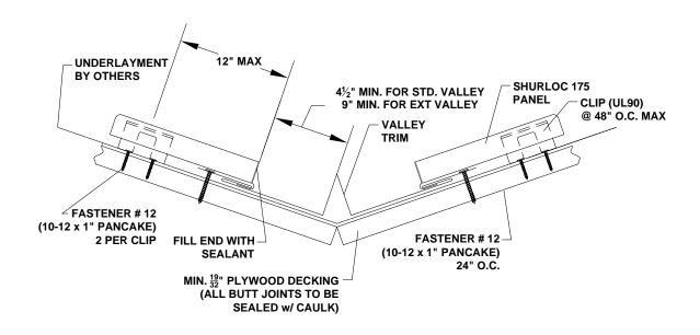
Figure 4: Valley Detail (Valley With Integrated Cleat)
