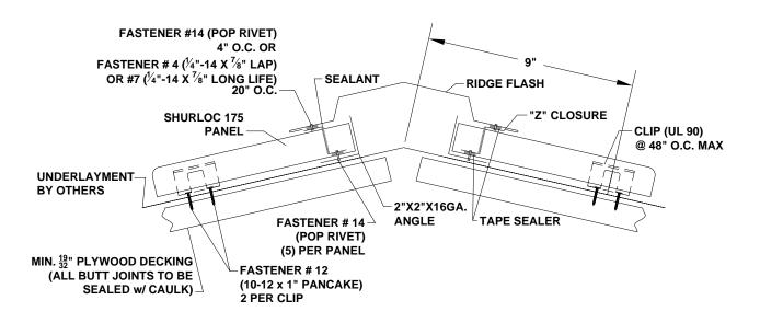
Figure 2: Floating Ridge/Hip Detail
