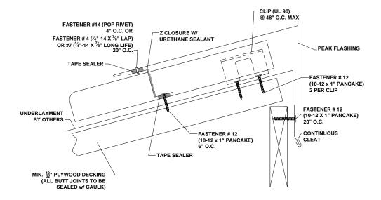
Figure 14: Fixed Peak Flashing Detail
