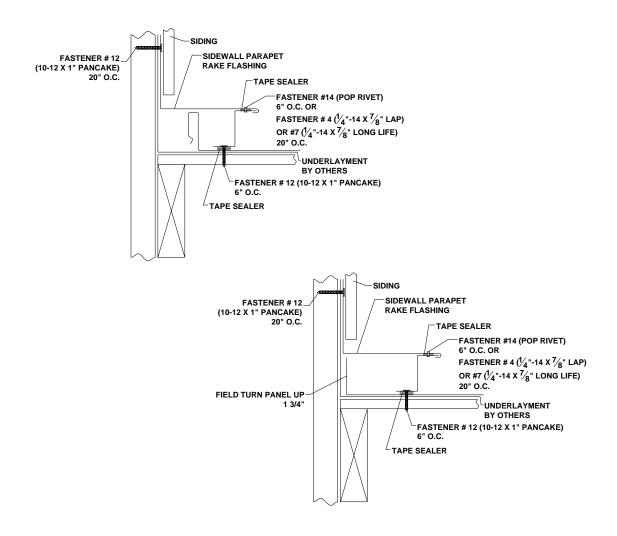
Figure 16: Sidewall/Parapet Fixed Rake Flashing Detail
