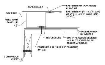
Figure 6: Fixed Rake/Gable Flashing Detail
