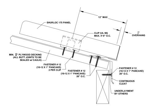
Figure 13: Alternative Eave Detail
