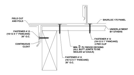
Figure 8: Alternative Rake/Gable Flashing Detail
