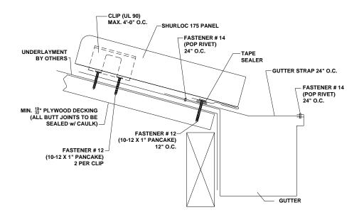
Figure 9: Gutter Detail
