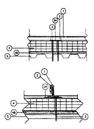
Metal Roof Deck Panels\* — No. 24 MSG min. Coated steel panels continuous over two or more spans. End laps to occur adjacent to purlins with panels overlapped 3 inch max. Side laps to be tightened and crimped with a special motorized crimping machine. A line of sealant may be used at panel end and side laps.
