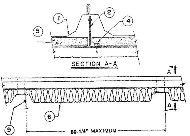
1. **Metal Roof Deck Panels\*** — For Class 90-No. 24 MSG coated steel, for Class 30-No. 26 MSG min. Coated steel panels continous over two or more spans. End laps to occur adjacent to (Item 7) or on top of (Item 7A) purlins with panels overlapped 3 inch max.). Side laps to be tightened and crimped with a special motorized crimping machine. A line of sealant may be used at panel end and side laps.
