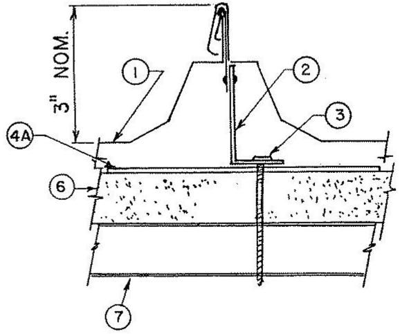
1. **Metal Roof Deck Panels\*** — No. 24 MSG min. Coated steel panels continuous over two or more spans. End laps to occur adjacent to purlins with panels overlapped 3 inch max. A line of sealant may be used at panel end and side laps. **A & S BUILDING SYSTEMS L P** (View Classification) — "Ultra-Dek"
