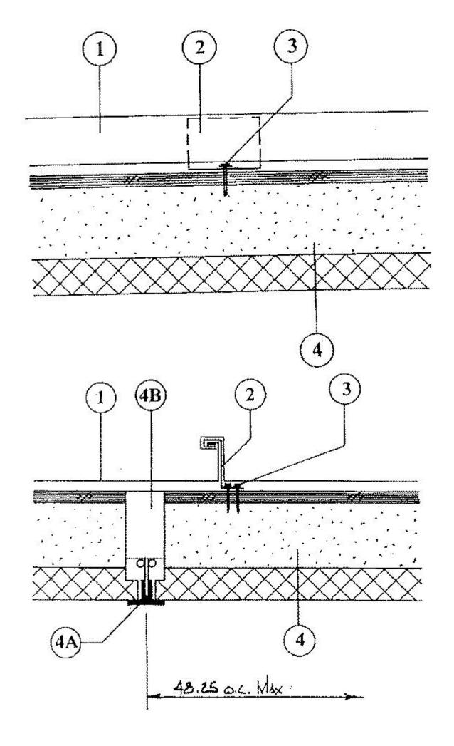
1. **Metal Roof Deck Panels\*** — 24 MSG minimum coated steel. Maximum panel width 16 in., and rib height 2 in. Panels continuous over two or more spans. Endlaps to occur with panels overlapped 6 in. A bead of sealant may be used at panel ends and side joints. Side laps to be tightened and crimped with an electric crimping machine to a maximum 45 degree angle unless indicated in the individual panels in this item. Crimping process to include the upper portion of panel clips (Item 2).
