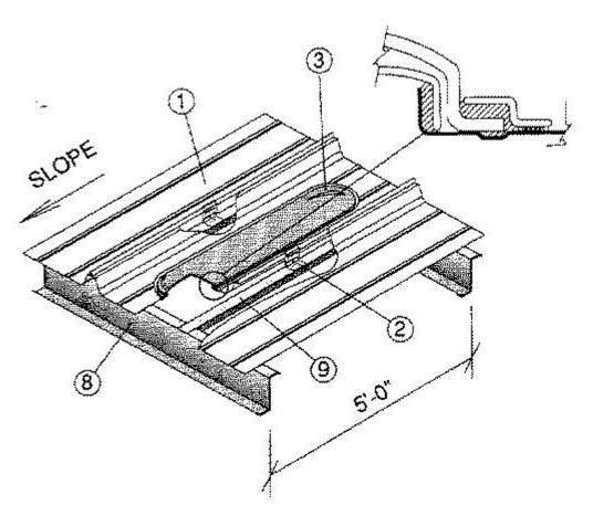
1. **Metal Roof Deck Panels\*** — No. 24 MSG minimum coated steel. Maximum panel width 24 in. Panels continuous over two or more spans. Endlaps to occur adjacent to purlin with panels overlapped 3 inches. A bead of sealant may be used at panel endlaps and sidelaps. Adjacent panels to be seamed together along side joints using an electric seaming tool. Seaming operation to include panel clip tabs (Item 2).
