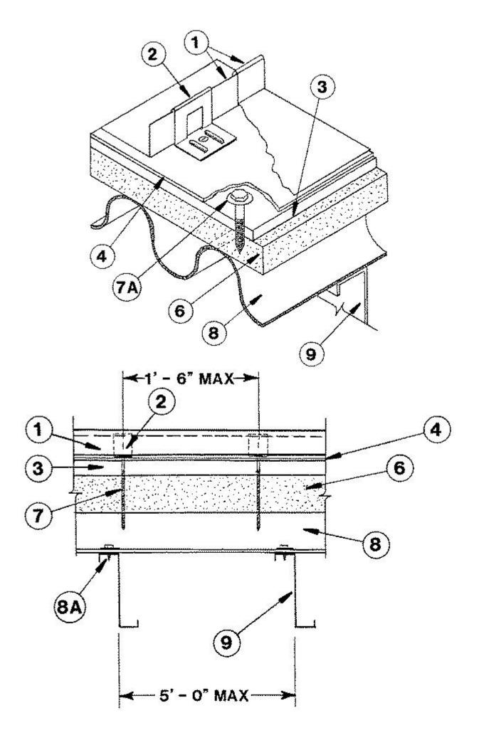
1. **Metal Roof Deck Panels\*** — No. 24 MSG min gauge coated steel. Panel width may be 20 in. or 12 in. Panel ribs to be 1-1/2 in. high at female side. Panels continuous over three or more clips with no end laps. **AEP SPAN, DIV OF ASC PROFILES** (View Classification) — "12 in. High-Seam", "20 in. High-Seam"
