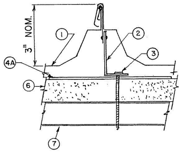
Metal Roof Deck Panels\* — 24 MSG min coated steel. Panels continuous over two or more spans. End laps to occur adjacent to purlin with panels overlapped 3 in. A line of sealant may be used at panel ends and side laps.
