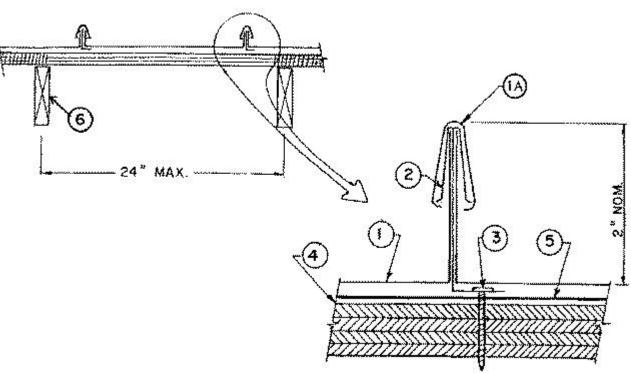
1. **Metal Roof Deck Panels\*** — No. 24 MSG min coated steel. Max panel width 22-1/2 in. and rib height 1-7/8 in. Panels continuous over two or more spans. End-laps to occur adjacent to supports with panels overlapped 4 in. A line of sealant may be used at panel ends and side laps.
